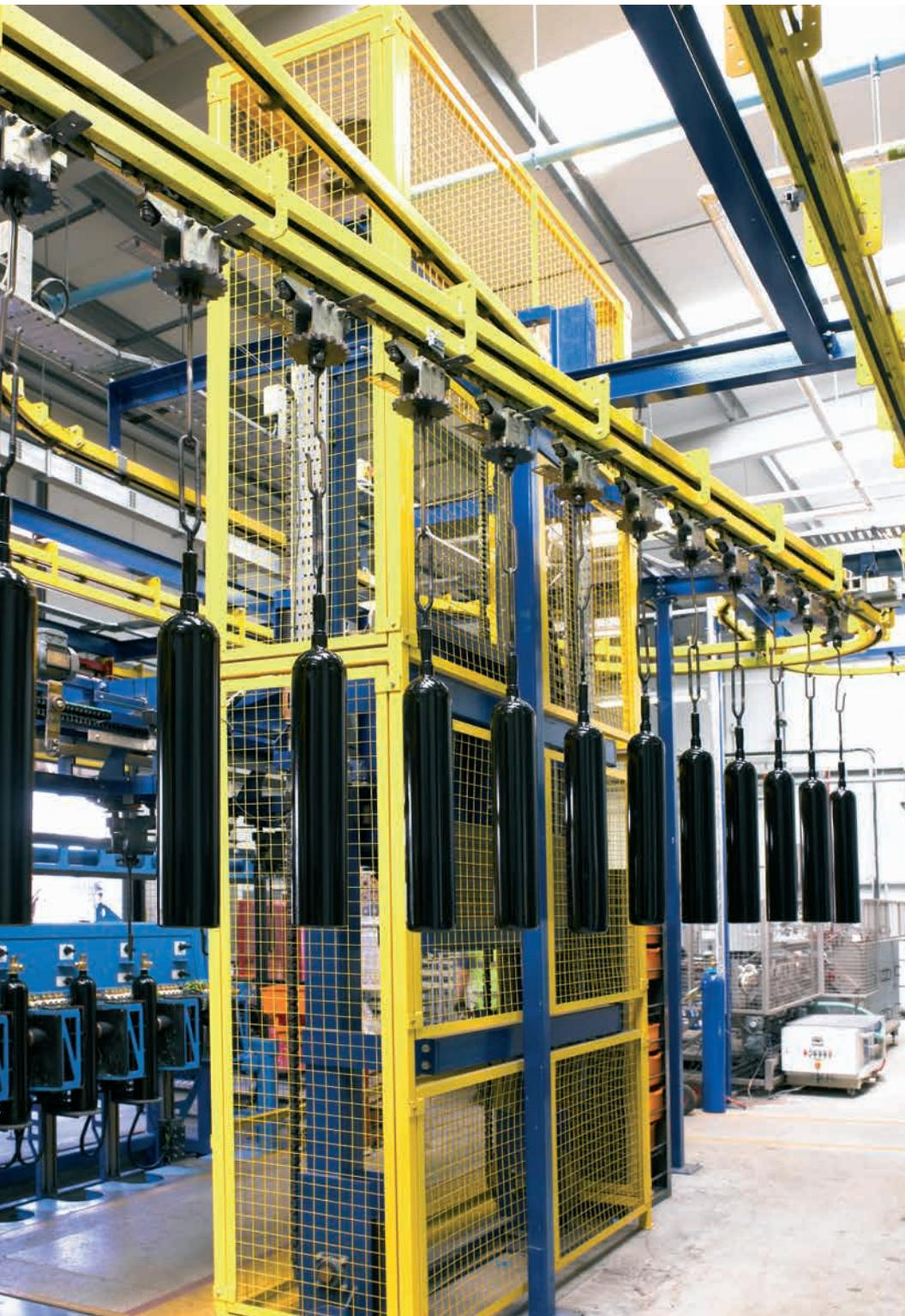
Leicester based LB Foster Materials Handling has installed a power and free overhead conveyor system in leading industrial gases company BOC's new state-of-the-art test centre in Wolverhampton.
